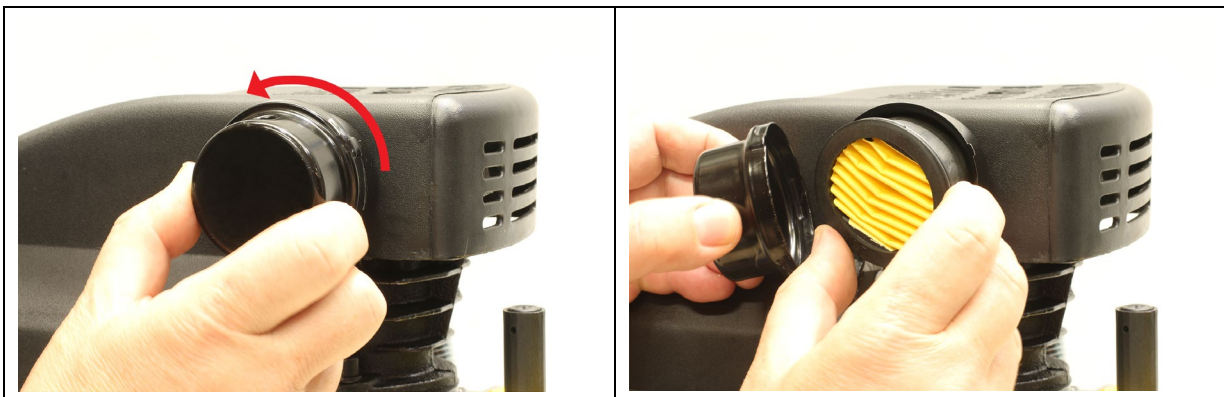
Figure 7-1 Air Filter Cover and Element Removal
